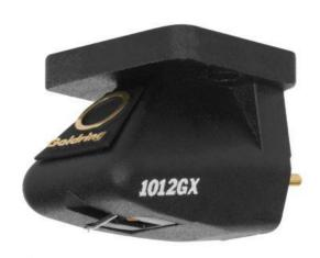
This hand-built cartridge uses the acclaimed Gyger II nude diamond stylus. A fine-line elliptical type with a 6  $\mu$ m small radius it gives smooth, extended highs, low distortion and reproduces a highly detailed and dynamic sound. Advanced diamond tip polishing ensures excellent tracking ability and reduces record wear. Because it fills the record groove more completely due to its larger major radius, the Gyger II represents a major upgrade over normal elliptical stylus types.
